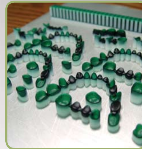
The ProJet™ DP 3-D Printer then generates the wax-ups.
